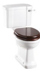
Rimless CC WC with 440 lever cistern W 440 D 730 H 780 Pan Height 420
